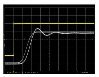
The smooth output waveform is from the SCS-817 Bessel filter, the step response with ringing is from the SCS-816 Butterworth filter.
